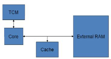
on-chip scratchpad RAM and some external off-chip RAM; it might be as complex as two or three levels of cache between the core and the external memory system.
